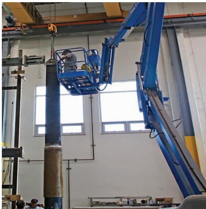
Testing of Simpson Strong-Tie® FX-70 Structural Repair and Strengthening System at Simpson's Tyrell Gilb Research Lab – the industry's first full-scale, cyclic test of a repaired wood pile.
