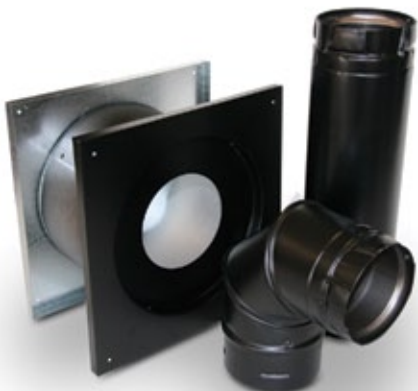
The PelletVent Pro line features pipe lengths manufactured on Dura-Vent's new laser welding equipment. The ability of the laser welder to produce a perfectly round tube enables us to offer a product that requires no sealants or gaskets.
