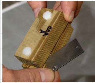
A small metal coupon is sandwiched between two blocks of pressure-treated wood and then placed in a humidified room to simulate elapsed time.
