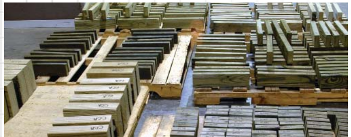
Different pressure-treated wood types fill pallet after pallet, waiting to be used for corrosion tests. All told, six different chemical treatments were tested.
