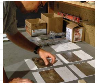
Simpson dedicated hundreds of hours to testing more than 5,000 coupons and screws made with 15 different metal finishes and coatings.
